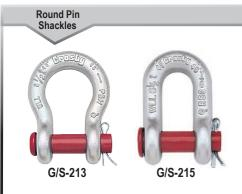
Round Pin Shackles can be used in tie down, towing, suspension or lifting applications where the load is strictly applied in-line. Round pin shackles should never be used in rigging applications to gather multiple sling legs, or where side loading conditions may occur.
