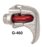
The Bundle Clip is utilized in a choker hitch application to maintain the shape of bundled packages after a load is placed. The Bundle Clip is attached to live line of choker hitch, but it is never to be used as a button or ferrule to carry a load in the primary load path.
