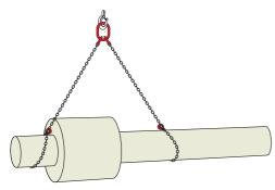
If the shape of the load permits it, the sling should be positioned equidistant about the centre of gravity ensuring a safe horizontal lift.
