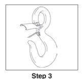
3. Position latch over tines of spring with ears partially over hook cam. Swing latch to one side of hook, point and depress latch and spring until latch clears point of hook.
