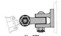
No. 576 Self-adjuster Fitting with Pad Jaw, King Pin, Tension Pin, Cup Spring and Washers.
