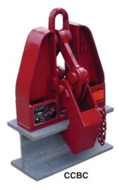
Crosby Clamp-Co<sup>®</sup> Beam Clamps provide an efficient method for handling wide flange beam sections and plate girders. When lifting, these beam clamps grip the beam at three points, and when properly balanced and safely guided, the beam can be handled even if the clamp is slightly off center lengthwise.
