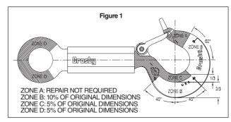
by grinding lengthwise, following the contour of the hook, provided that the reduced dimension is within the limits shown in Figure 1. Contact Crosby Engineering to evaluate any cracks.
