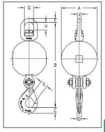
**UB-550E Top Swivel Overhaul Balls with Crosby Eye Hook**
