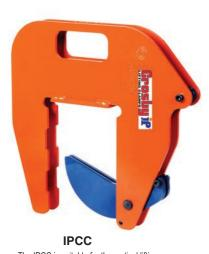
The IPCC is suitable for the vertical lifting and transfer of concrete pipe sections and wells. Very easy application and removal of the clamp thanks to the built-in carrying-grips. Normally used in combination with 7mm chain (not supplied). These clamps must be used in pairs or more.
