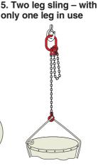
WLL: Rate at half the working load marked on the sling. The WLL should be no more than 80% if used in choke hitch.
