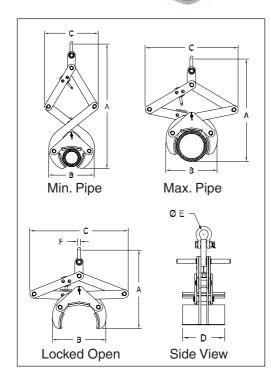
The new Crosby Clamp-Co® Adjustable Pipe Grab provides an excellent means of handling cylindrical objects. Featuring padded grabs, the new Grab offers an excellent method of handling any pipe or solid bar, 3.5" to 36", especially where damage to material surface is not permitted.
