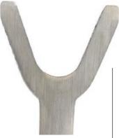
Unretouched photograph of a section cut from a flame hardened McKissick sheave (etched 2-1/2 Minutes).
