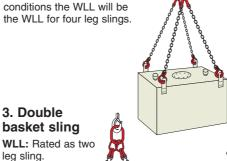
Comment: This WLL applies to double basket slings designed as such and fitted with a KUPLEX Master Assembly strong enough for this duty. It does not apply to a back-hooked two leg sling. The maximum included angle should be 90° measured between diagonally opposite legs, or maximum 45° from vertical.
