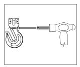
Step 1: Using a hammer and the correct roll-pin punch per chart on the right, drive the old latch pin assembly out of hook.
