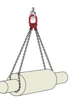
**WLL:** Rate as a two leg sling. The angle of any leg should not exceed 45° from the vertical
