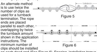
on each dead end (See Figure 6). Spacing, installation torque, and other instructions still apply.
