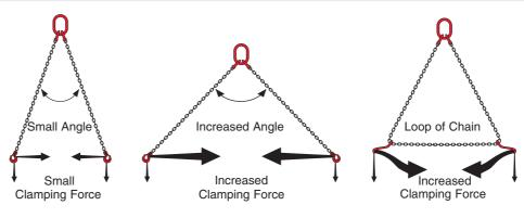
The slinger should be aware of this force so that he may use it to his advantage and avoid the dangers which it might cause. For example, with this shape of load, the clamping force is used to good effect in ensuring that the hooks are clamped tightly against the load. A minimum of 60° included angle is required (30° to vertical).
