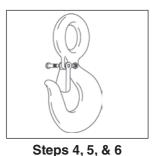
4. Line up holes in latch with hook cam.
