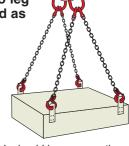
**WLL:** The WLL should be no more than that applicable to an equivalent four leg sling.
