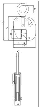
Model IPBUUZ: with Universal Hoisting Eye Model IPBUZ: with Fixed Hoisting Eye ———
