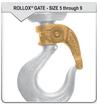
**To Lock:** Close the gate; a stainless steel pin is mounted in a horizontal bore which passes through the gate and engages a notch milled in the hook shank.
