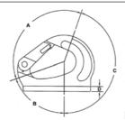
ZONE A: REPAIR NOT REQUIRED (LATCH EXCLUDED) ZONE B: 10% OF ORIGINAL DIMENSION ZONE C: 5% OF ORIGINAL DIMENSION ZONE D: ONLY AREA ALLOWED TO BE WELDED
