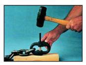
Drive the pin through the assembled link ends and sleeve until the end of the pin is flush with the outside of the connecting link halves.
