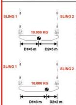
WHEN LIFTING VERTICALLY, THE LOAD WILL BE SHARED EQUALLY IF THE SLING 2 CENTER OF GRAVITY IS PLACED **EQUALLY BETWEEN THE PICK POINTS.IF** THE WEIGHT OF LOAD IS 10.000 KG, THEN EACH SLING WILL HAVE A LOAD OF 5,000KG AND EACH SHACKLE AND EYEBOLT WILL ALSO HAVE A LOAD OF
