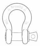
**SCREW PIN** Use when picking and placing a load, tighten pin prior to each lift.
