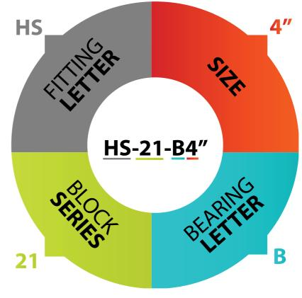
If blocks are not shown with type of fitting you require, simply choose letter corresponding to your fitting need and insert where "HS" appears in the above example.
