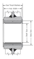
Roller Bearings without inner races are designed to operate on shafts carborized to 60 Rockwell C and grounded to +/- .0005 of shaft size.
