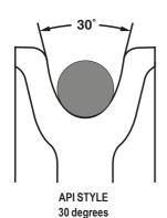
The sheave profile is a very important feature of all sheaves. McKissick manufactures standard sheaves for general use in hoisting Wireline guide applications to minimal API Specifications. The profile includes included groove angle of 30°. This groove profile is used in mobile cranes, drilling rigs, working units, tubing blocks, traveling blocks, crown blocks and many other general hoisting applications.
