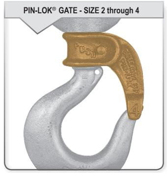
**To Lock:** Close the gate; a stainless steel pin is carried in a horizontal bore and engages a milled slot in the hook shank.
