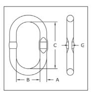
A-344 Welded Master Links with Engineered Flat
