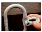
Slide Coupler Link over Engineered Flat of Master Link.
