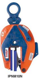
The IPNM10N vertical lifting clamp is used for lifting, turning, moving or vertical transfer of sheet, plates, or fabrications from horizontal to vertical and down to horizontal (180°) as needed without marring the surface of the material. Materials such as aluminum, stainless steel, painted materials, aircraft skins, composite material, glass, plastic, etc., can be lifted without marring.
