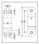
The Crosby AS-17 Slurry Swivel is a zinc plated Bullet Type Swivel (AS-7), designed with two rubber lip style seals about the shaft. The threaded cap is sealed with a silicone sealant and secured with a set screw. The swivels are provided with an Alemite grease fitting for easy lubrication.
