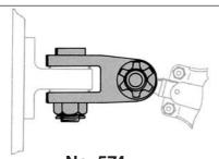
No. 574 Self-adjuster Fitting with Tension Pin, Cup Spring and Washers, and King Pin to fit Pad Eye (can also be furnished with 2 Tension Pins).
