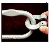
Rotate Coupler Link so that clevis fitting is to the outside of Master Link and attach to chain sling.
