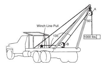
There is no mechanical advantage to a single part load line system, so winch line pull is equal to 1,000 kg or the weight being lifted.
