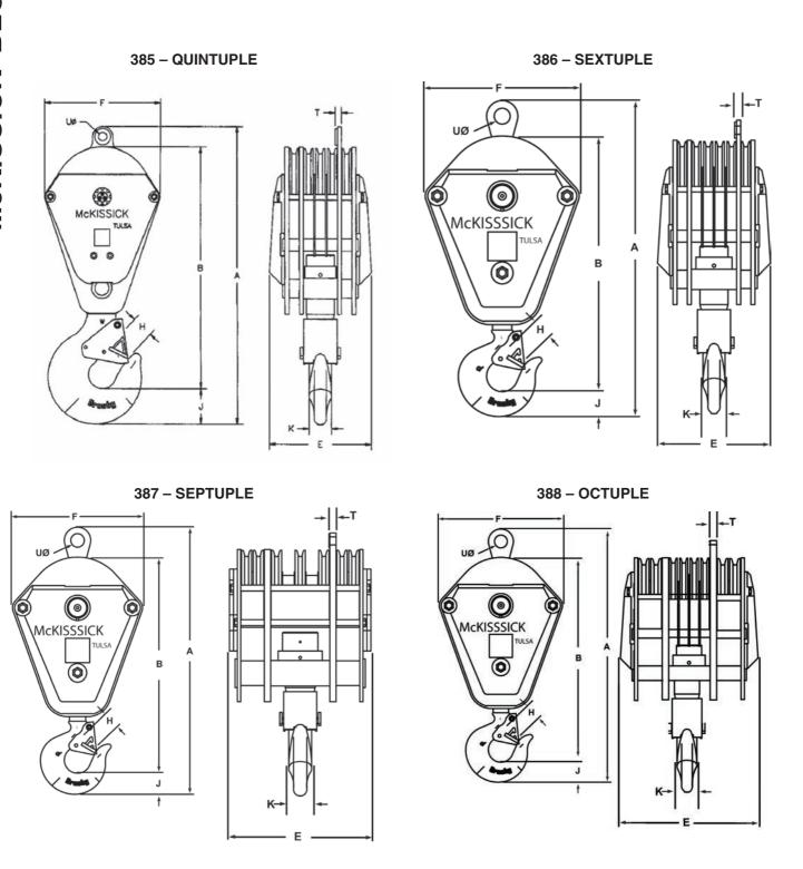
Thickness (E) shown is for blocks containing cheek weights (Light Medium - LM, Medium - M, and Heavy - H).
