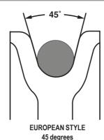
DIN 15061 lifting appliances defines groove profiles for Wireline sheaves.
