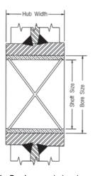
Roller Bearings are designed to operate on shafts carborized to 60 Rockwell C and grounded to +/- .0005 of shaft size.
