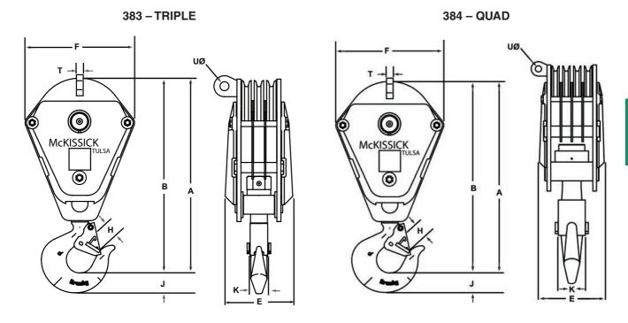
Thickness (E) shown is for blocks containing cheek weights (Light Medium - LM, Medium - M, and Heavy - H).
