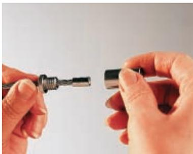
Montage mittels ASS Zylinderterminal
